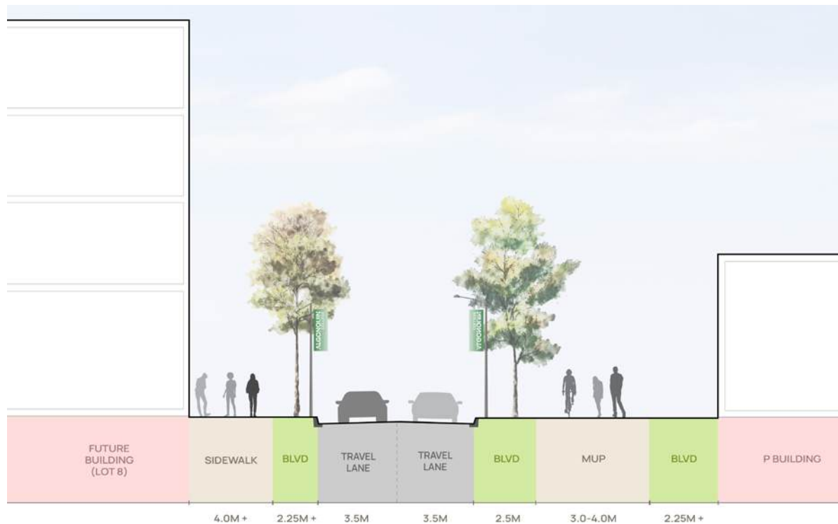
Figure 13. Wàbisheshì Cross Section Looking East
