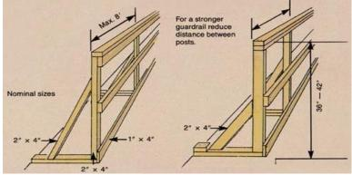
Wood guardrails must be supported by posts extending to the top rail and braced and solidly fastened to the floor. Shoring jacks used, as posts should be fitted with plywood softener plates at top and bottom. Snug up and check the posts regularly for tightness.
