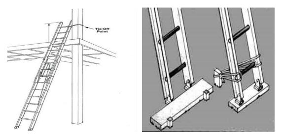
The top of the ladder should extend at least 3 ft. (.9m) above the landing to provide a hand hold for getting on and off of the ladder. If needed, secure the top of the ladder. Tie the top of the extension ladder to an anchor point.
