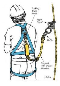
Employees exposed to a free fall distance of 3 m (10ft) or more (without restraint) must wear fall arresting equipment, using a full-body harness system. Inspect components of the fall arrest system before each use for wear, damage and other deterioration. Defective components are removed from service when the components' function or strength has been adversely affected.
