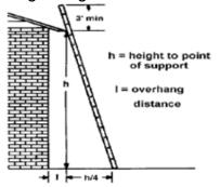
Extension ladder should be secured at the top or bottom to prevent movement. The base of an extension ladder must be secured in place by using the safety feet on the ladder or by other means.
