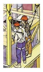
Look for cuts, fraying, broken stitching, and other damage to webbing. Check for chemical or heat damage.
