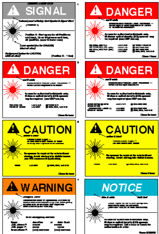
Figure A-1 Displays a generic sign with the following general characteristics (from top to bottom): at the top is a colored signal-word panel with a safety-alert symbol (exclamation point within an equilateral triangle) and a signal word; below this is a word message designated as Position 1; this is followed by a graphic symbol (in this case, a laser-sunburst symbol); positions 2 and 3 are final word messages. Older signs that conformed to ANSI standards shall remain
