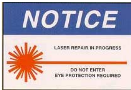
Fig. 6 (ii)- Sample Temporary Laser Controlled Area sign. This sign shall be posted outside a temporary controlled area, for example, during periods of service. The area outside the temporary controlled area remains Class 1, while the area within is either Class 3b or 4.
